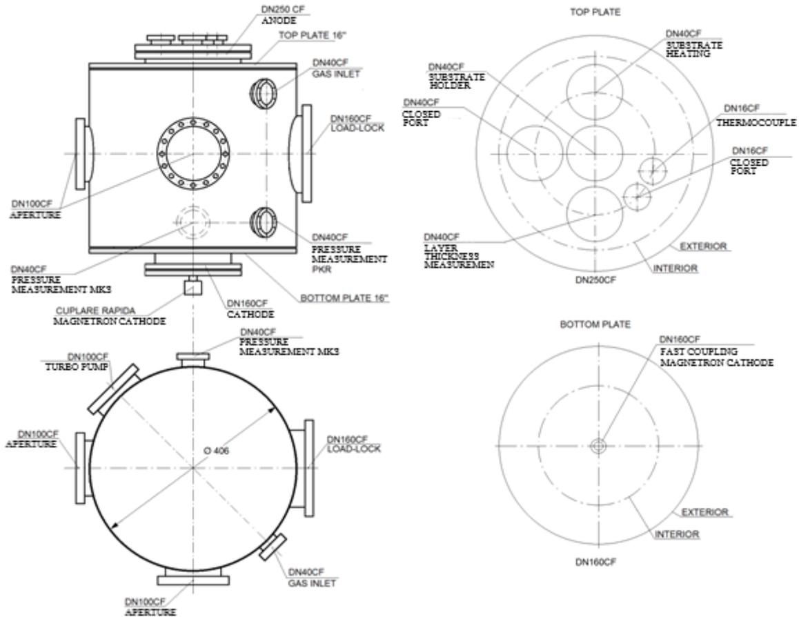
**Figure 1.** Vacuum chamber design.
