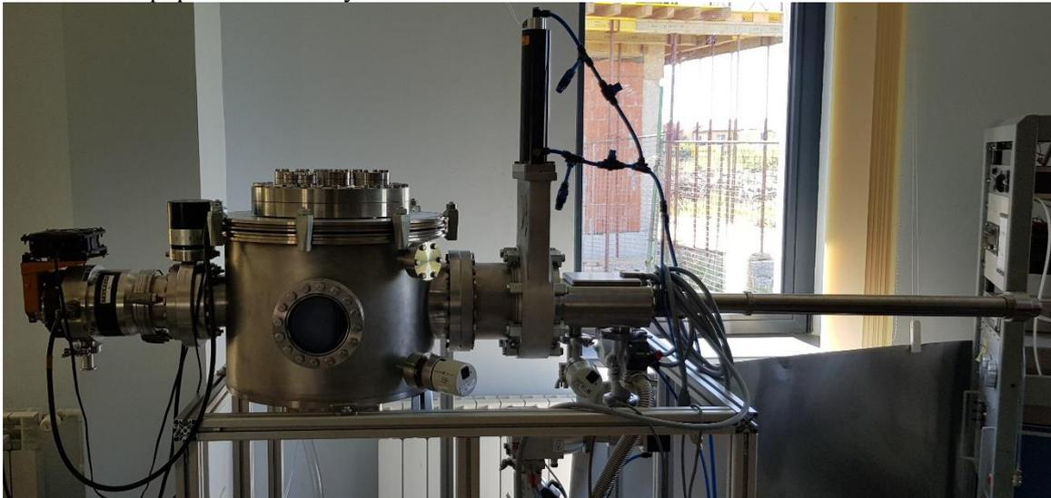
**Figure 3.** Vacuum chamber with sensors, load-lock, and vacuum pump
